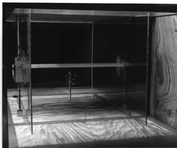
Fig. 10 Photograph of the testing arrangement with splitter plates.
